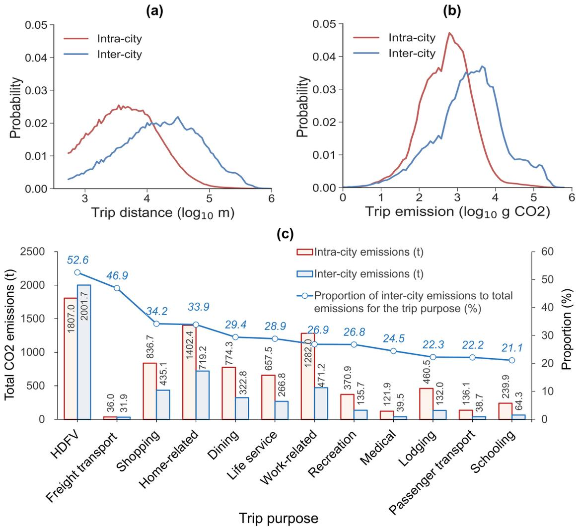
Figure 5: Statistics of road CO<sub>2</sub> emissions from intra-city and inter-city trips. (a) Probability distribution of trip distances (logarithmic scale) for intra-city and inter-city trips. (b) Probability distribution of CO<sub>2</sub> emissions (logarithmic scale) for intra-city and inter-city trips. (c) Total road CO<sub>2</sub> emissions of intra-city and inter-city trips and the proportion of inter-city emissions to total emissions for each trip purpose.
