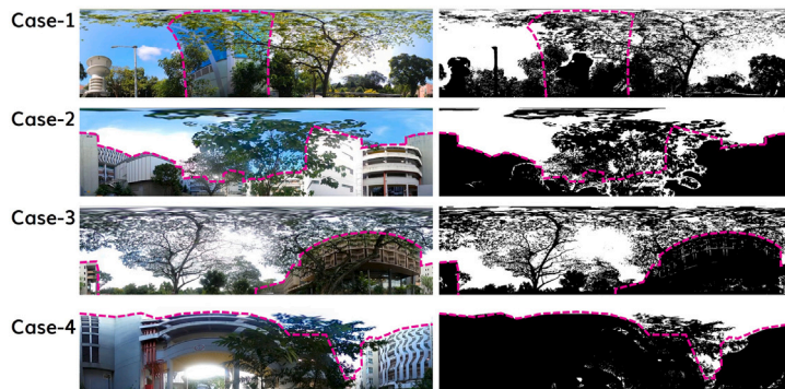
Fig. 20. Example results of binarization applied to panoramic imagery featuring buildings obscured by tree canopies. Pink dashed lines indicates manually drawn edges between the buildings and background.
