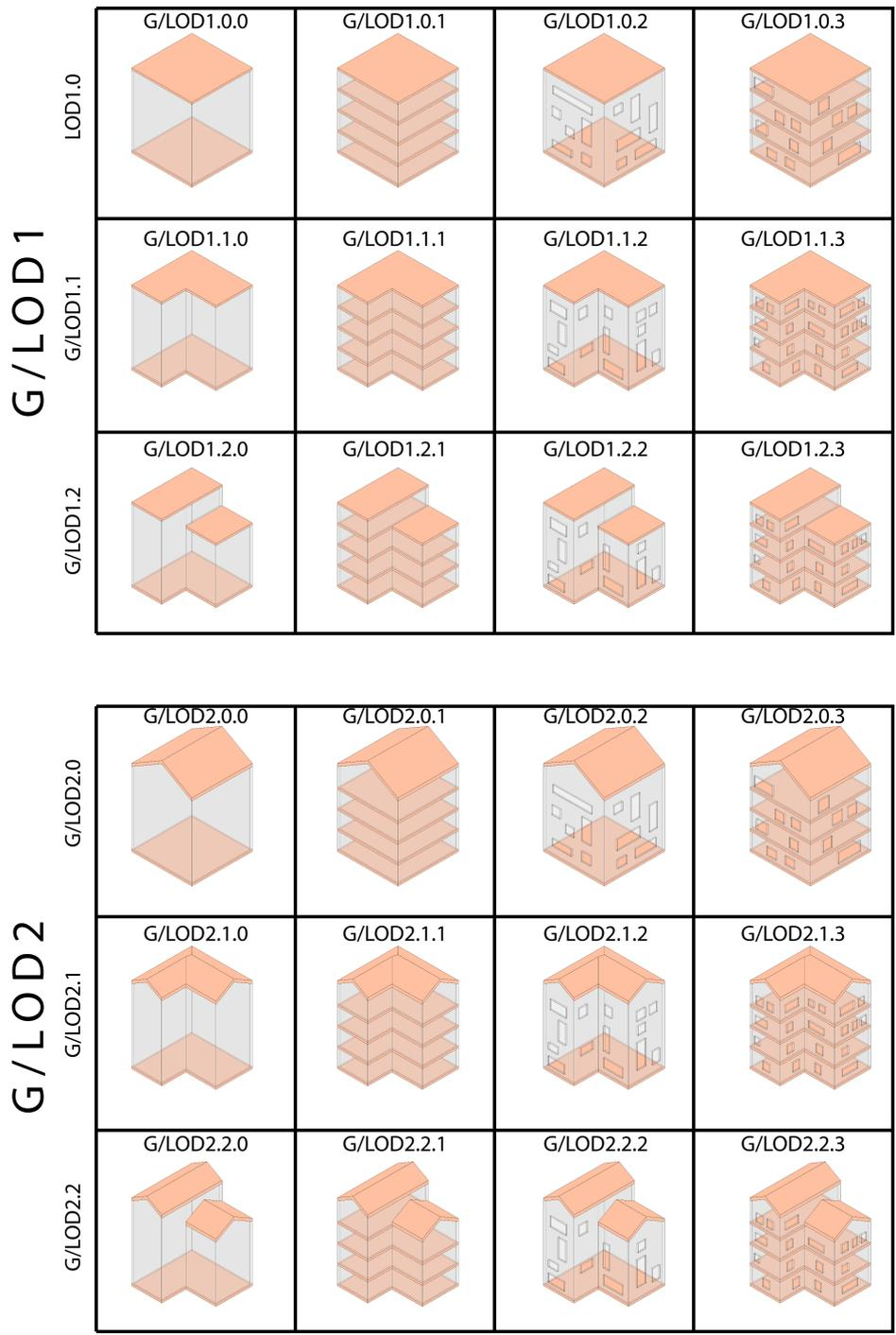
Figure 2: Levels of Detail for geometries used in urban energy modeling literature (Detailed explanations for each acronym can be found in Appendix A.)
