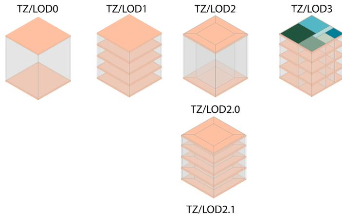
Figure 1: Levels of Detail for thermal zone layer used in urban energy modeling literature(Detailed explanations for each acronym can be found in Appendix A.).
