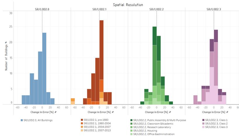
Figure 12: How the annual simulation error improved and worsened for the buildings based on aggregation approach.
