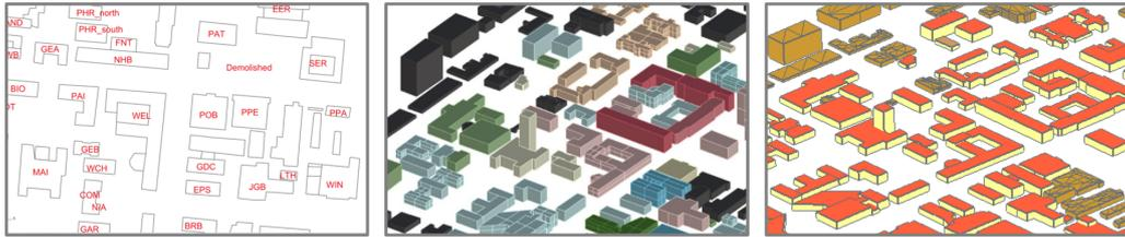
Figure 5: Example of creating UBEM (from left to right, the whole process of creating CitySim model, openings such as window to wall ratio have been assigned in the xml file; thus they are not visible on the graphics).
