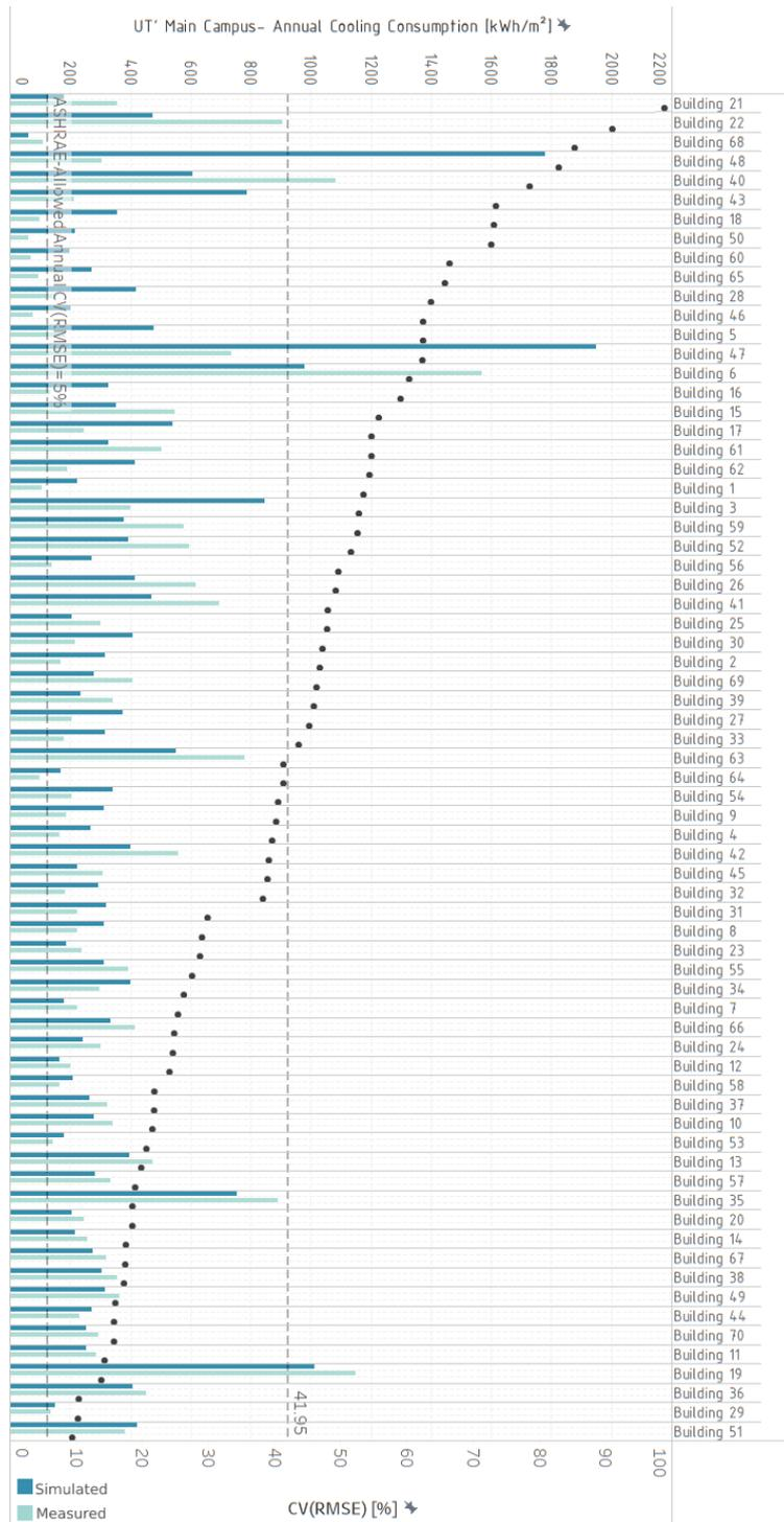
Figure 8: CV(RMSE) of each building before Bayesian Calibration at Annual Temporal Resolution (TR/LOD0).
