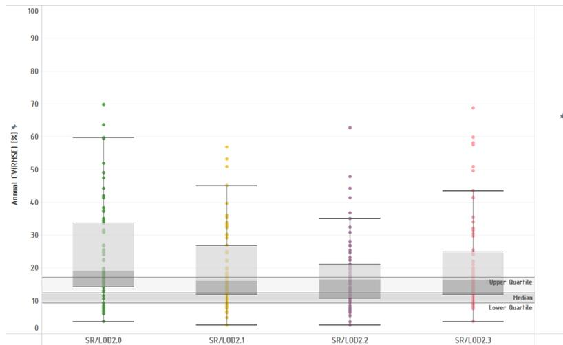
Figure 13: Annual CV(RMSE) distribution after Bayesian Calibration performed against annual cooling data compared to the building level error for 70 Buildings.
