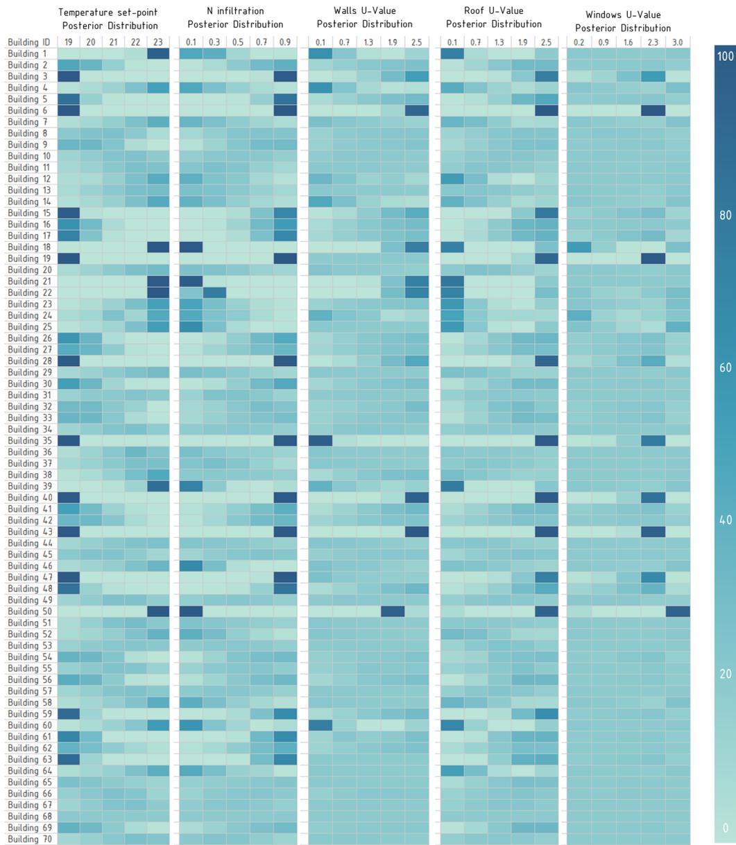
Figure 7: Marginal posterior distribution of Maximum Temperature set-point, Infiltration rate, Walls U-value, Roof U-value, and Window U-Value visualized in a heat map. Each row represents one building, and color intensity represents probability (%). The prior distribution is constant as 20% for given inputs. Calibration is performed by using each building's annual cooling consumption data available for three years.
