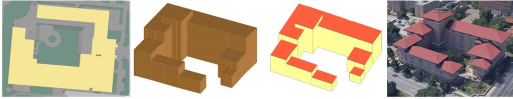
Figure 4: Sample campus building represented with (a) Building Footprint and (b) 3D Model in Rhino, (c) CitySim Energy Model (G/LOD1.2.2 and TZ/LOD0) in comparison to (d) a Google Earth view.
