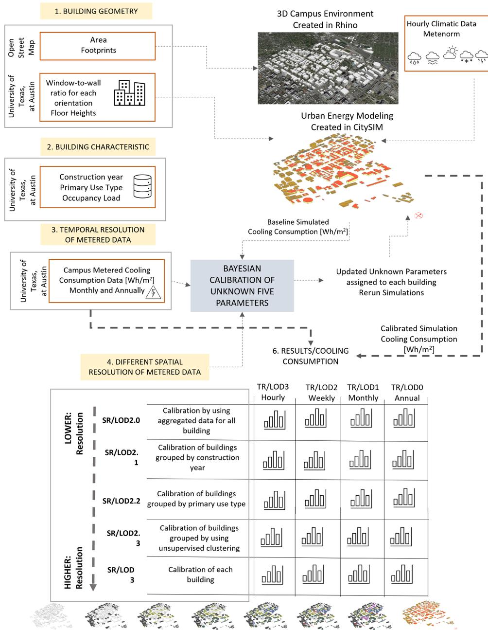
Figure 3: Schematic of the Bayesian Calibration and Modeling Process.
