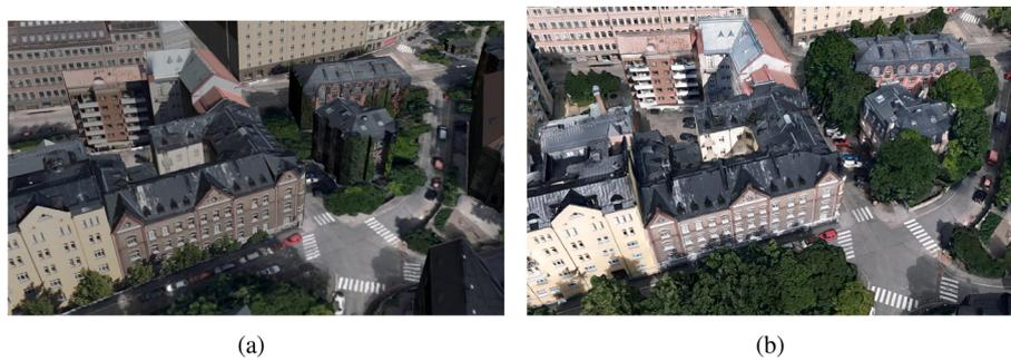
Fig. 4. 3D building models used in our work: (a) reality mesh models, used for training; and (b) semantic LoD2 models, which we use in the evaluation. Source of data: City of Helsinki.
