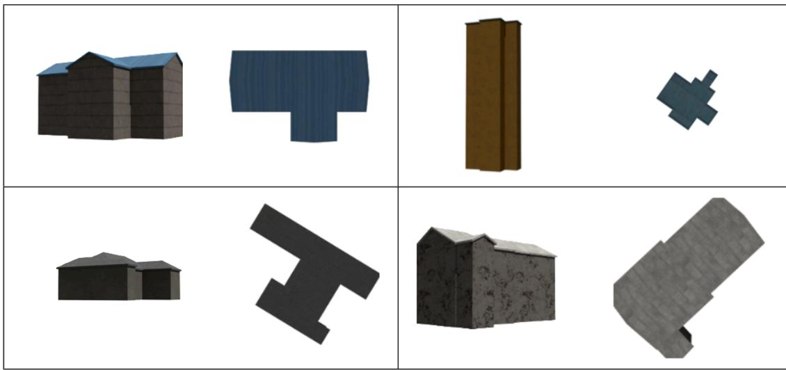
**Fig. 6.** Examples of building models generated from our pipeline that relies on modified open-source software, together with their side and top views used for training and testing.
