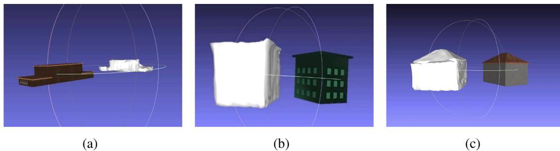
**Fig. 15.** Trained model was able to predict buildings (a) of non-uniform height (b) containing overhangs and (c) of non-flat roof types (Scenario 2).
