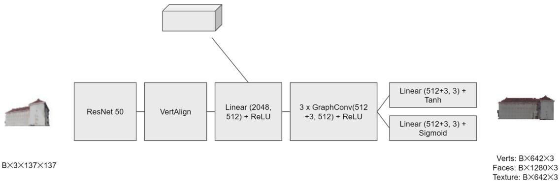
**Fig. 10.** Modified Pixel2Mesh model architecture to take in a single side-view and an initialised block mesh for refinement.
