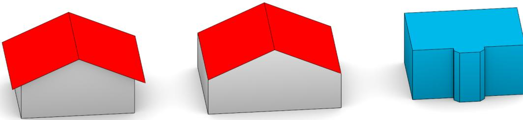
Figure 2: Two variants of LOD2 and an LOD1 model exposing the shortcomings of the CityGML LOD concept, and why the computer graphics principles cannot be fully applied to GIS and 3D city modelling.
