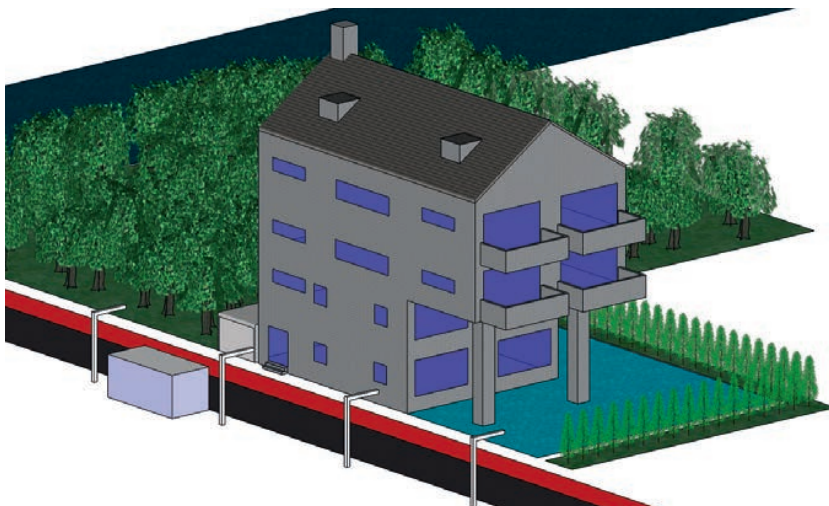
▲ Figure 4, Depiction of LOD6 and LOD7 models in the refined series of LODs.
