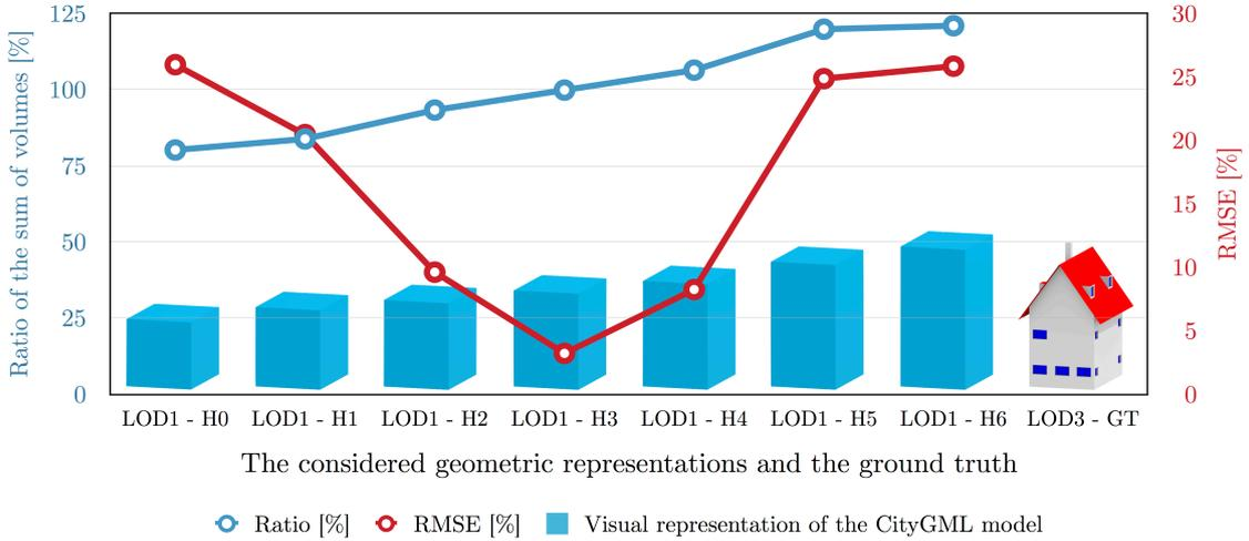
Figure 3: Results of the computation of volumes with the errors depending on the used geometric representation.
